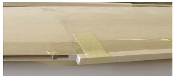
19. Carefully plane/sand both rear spar and leading edge to shape. Tip: when using David Plane set blade at slight angle so that the cut is thinner on one side of the plane. It helps control thickness of cut.
