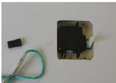
8. Centre Aileron servos using transmitter sub-trim and adjust Aileron pushrods. When satisfied tape servo covers in place.
