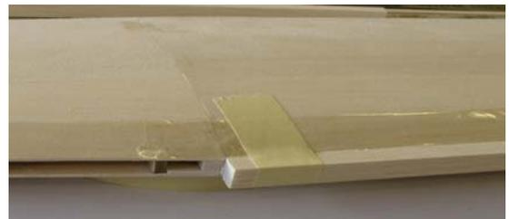
18. Carefully plane/sand both rear spar and leading edge to shape. *Tip:* when using David Plane set blade at slight angle so that the cut is thinner on one side of the plane. It helps control thickness of cut.
