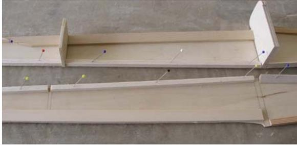
15. Glue strip longeron super structure to the fuselage sides.
