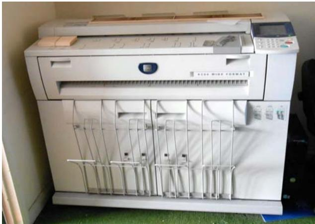
Digital AO Laser Plan Printer/Copier/Scanner
