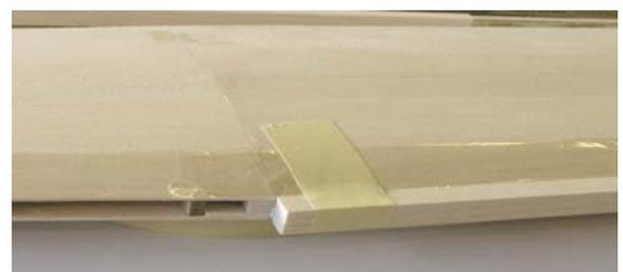
19. Carefully plane/sand both rear spar and leading edge to shape. Tip: when using David Plane set blade at slight angle so that the cut is thinner on one side of the plane. It helps control thickness of cut.
