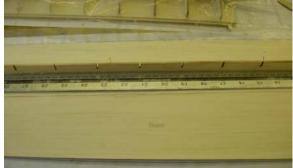
3. Accurately align the bottom sheeting on the plan with the wing trailing edge. Note the front
